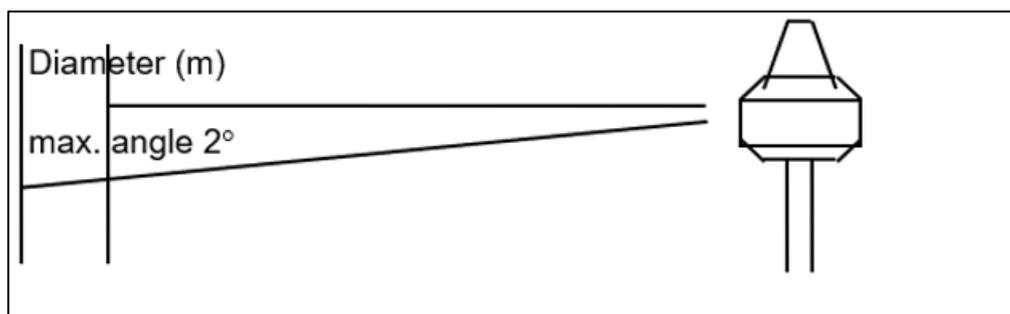
If two Inmarsat-C antennae are installed the vertical distance between them should be at least 1 metre to eliminate interference.
